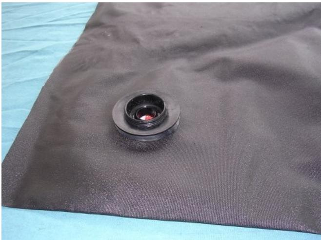
Put in the inflator. Fill the bag with water and leave it for a while. The leftover paper will be easier to clean out that way
