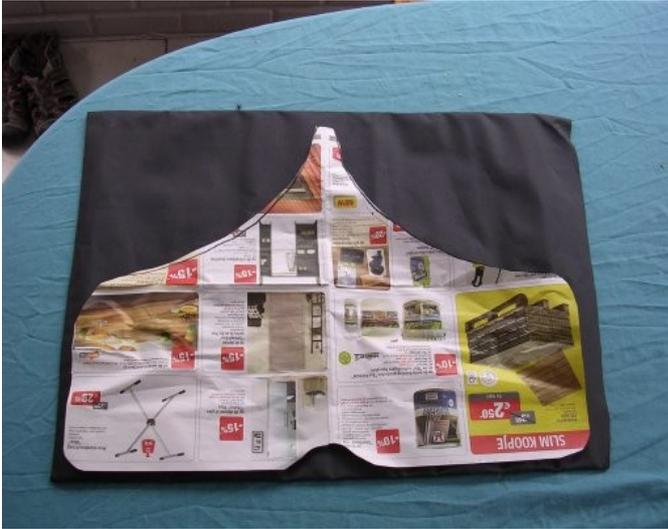
Put the papper inside the bag and iron the bag with the metal plate underneath. Make the bag really hot. When its hot lightly hammer the edges of the bag.
