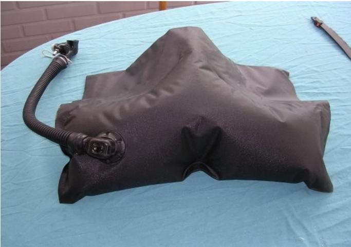
Clean out the leftover paper and fill the bag with air. You can now pressure test it by standing on the bag. If the overpressure valve kicks in the seals are strong enough. If not you need to redo the seal with the heating Iron.
