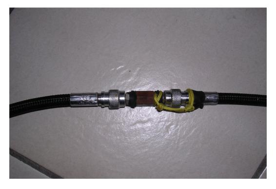
This manifold was tested to -40m. But became hard to breathe from -30m. It might be an aid in some situations but needs to be practised and tested prior to use.
