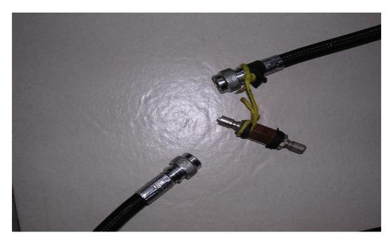
This small thingy lets you connect any two standard inflator hoses together to create a low pressure manifold. Provided the IP of both first stages is equal.
